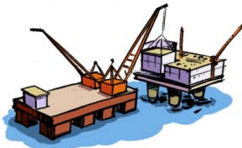
Figure 9.3 Principle of Topsides Removal
