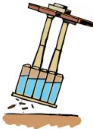
Figure 9.17 Tilt During Lift-off from the Seabed Causing Differential Water Pressure on some Inner Walls
