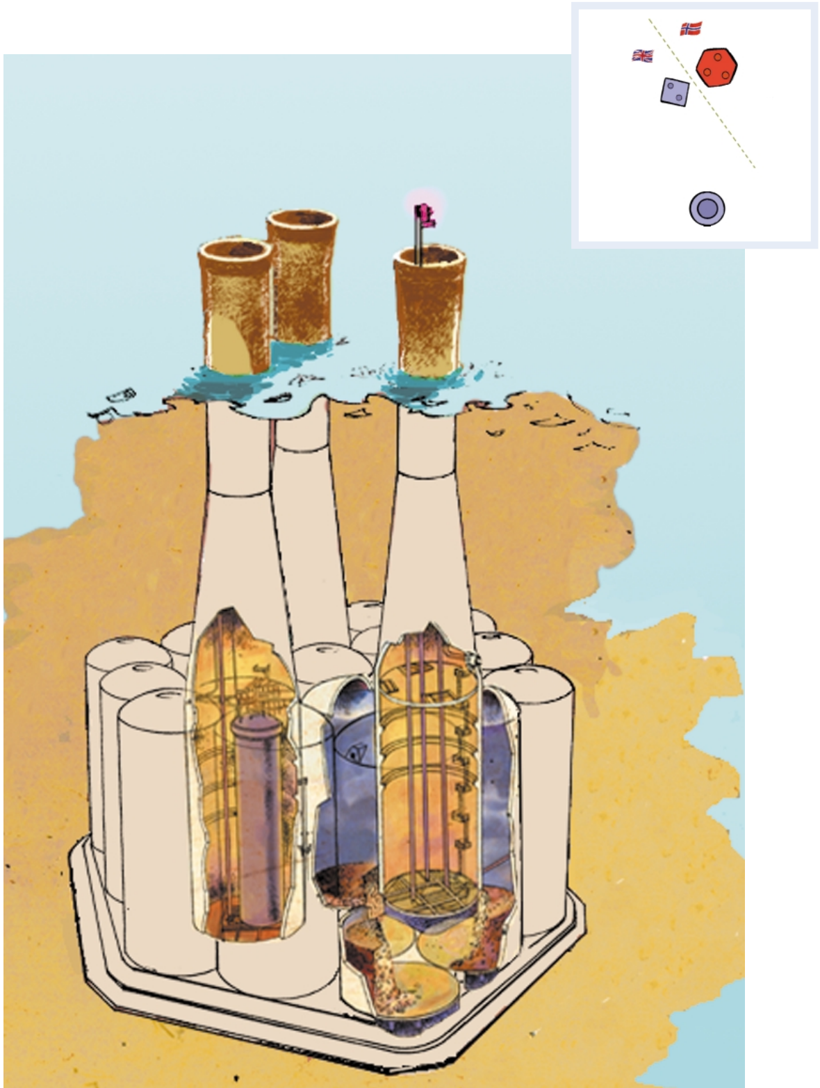
Figure 4.1 Concrete Substructure of Treatment and Compression Platform 2 (TCP2)
