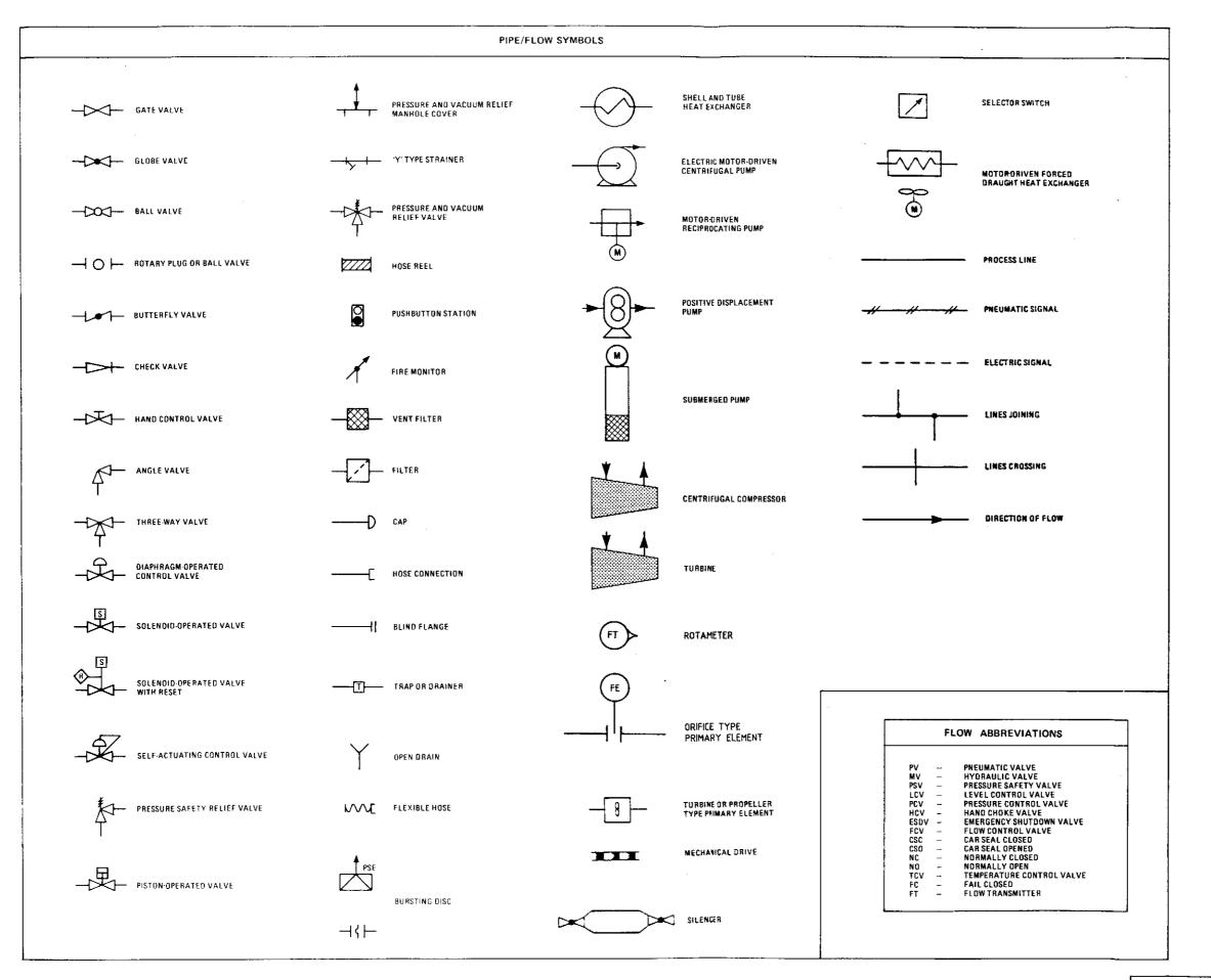
INSTRUMENT SYMBOLS PI PRESSURE INDICATOR PT ) PRESSURE TRANSMITTER (LC) LEVEL CONTROL ( LSL ) LEVEL SWITCH LOW (LSLL) LEVEL SWITCH LOW LOW (LSH) LEVEL SWITCH HIGH (LSHH) LEVEL SWITCH HIGH HIGH ( TI ) TEMPERATURE INDICATOR ( TT ) TEMPERATURE TRANSMITTER ( PC ) PRESSURE CONTROLLER PIC PRESSURE INDICATOR CONTROLLER OIFFERENTIAL PRESSURE INDICATOR ( FIC ) FLOW INDICATOR CONTROLLER ( LI ) LEVEL INDICATOR (FT) FLOW TRANSMITTER
